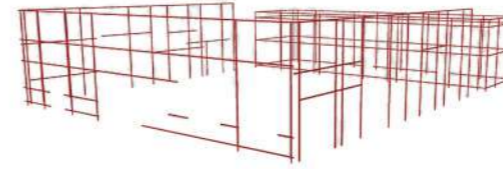
SUPPORT STRUCTURE THIS GRID SYSTEM OF STEEL BEAMS ACT AS THE SUPPORT SYSTEM FOR THE CORRUGATED IRON SHEETS.
