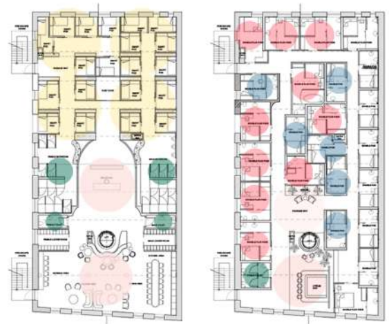
ZONING: PUBLIC AREAS WC / TOILETS SMART POD DOUBLE POD DOUBLE PLUS POD
