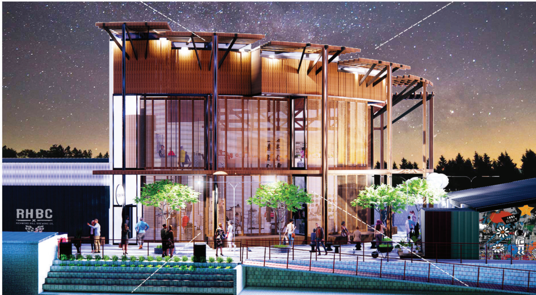
Water flows through Channels on the Roof, down pipes that run parallel to the elevator shaft and is then stored and harvested from rainwater tanks located beneath the raised flooring
