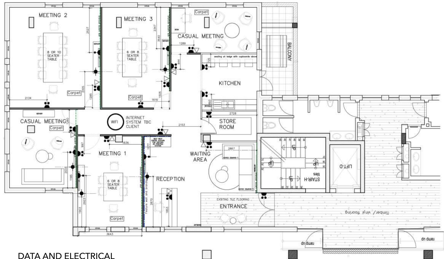
DATA AND ELECTRICAL SCALE | NTS
